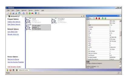
The Solutions-D software provides a way to configure many products in the 777 family of overload relays and power monitors, and with activation can be used to monitor and configure most DeviceNet<sup>™</sup> devices.
